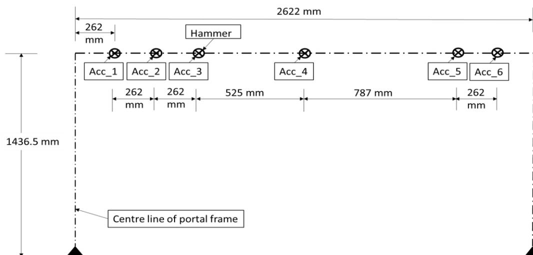
Figure 4. Location details of accelerometers and impulse hammer
