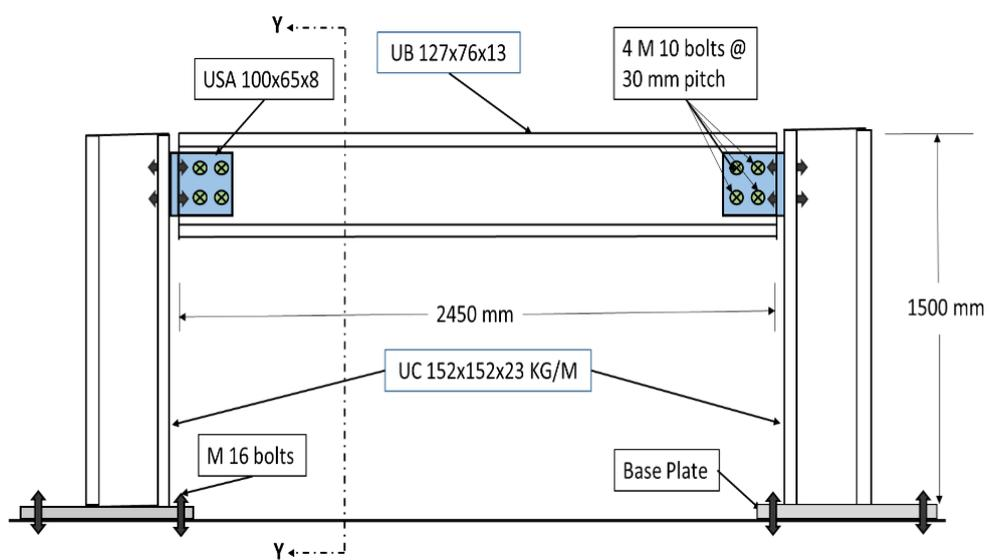
Figure 2. Frame components and connection details
