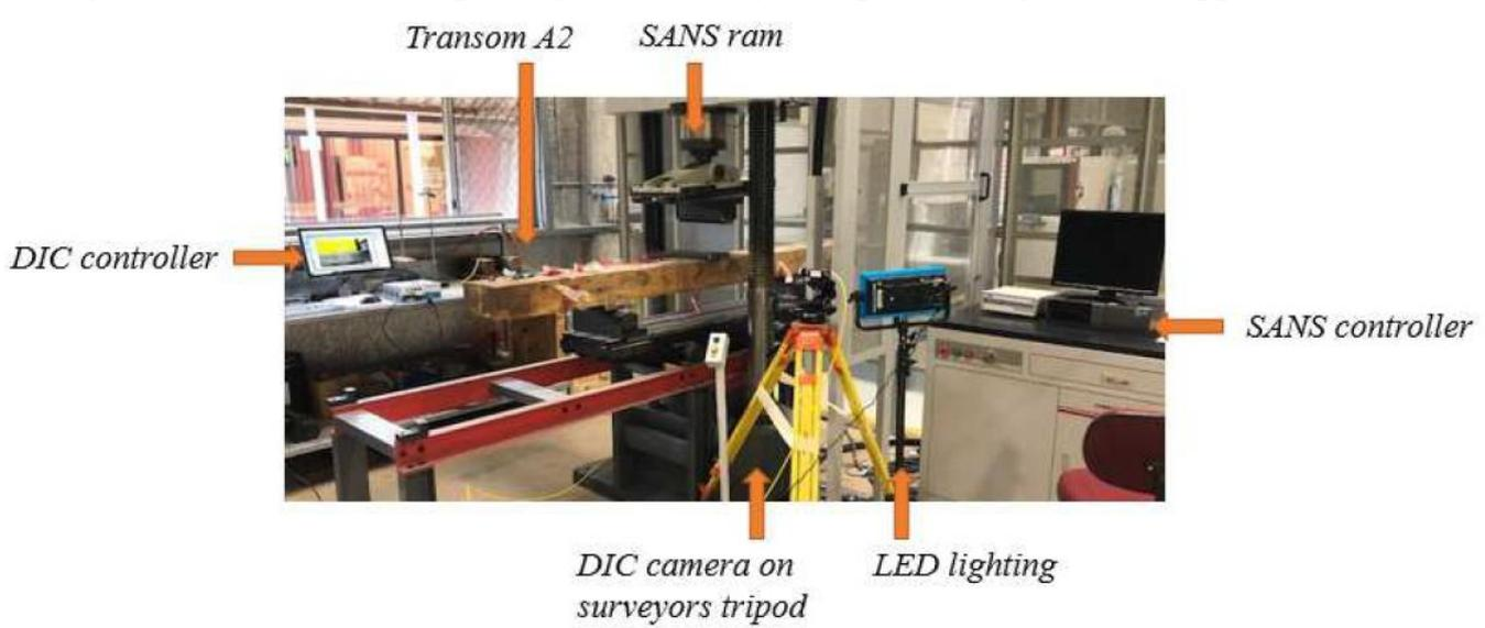
**Figure 2.** Lab trial of CFM’s DIC system
