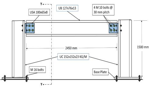
Figure 2. Frame components and connection details
