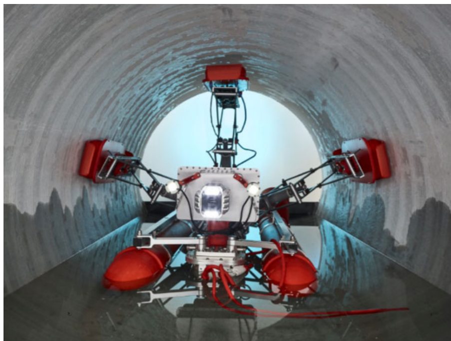
Figure 2. In-pipe sensing robot for condition assessments of concrete wastewater pipes [8].
