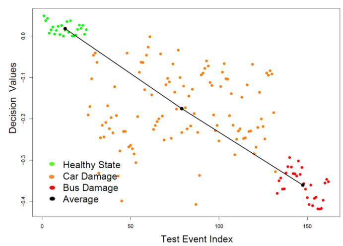
Figure 6. Damage identification results using tensor feature (Anaissi et al, 2018).
